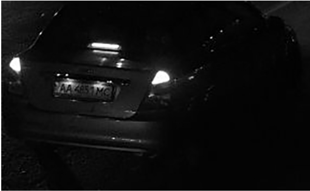
Fig. 17: Insufficient light to recognize license plate
