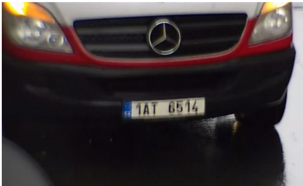
Fig. 14: Blurred license plate due to long exposure time
