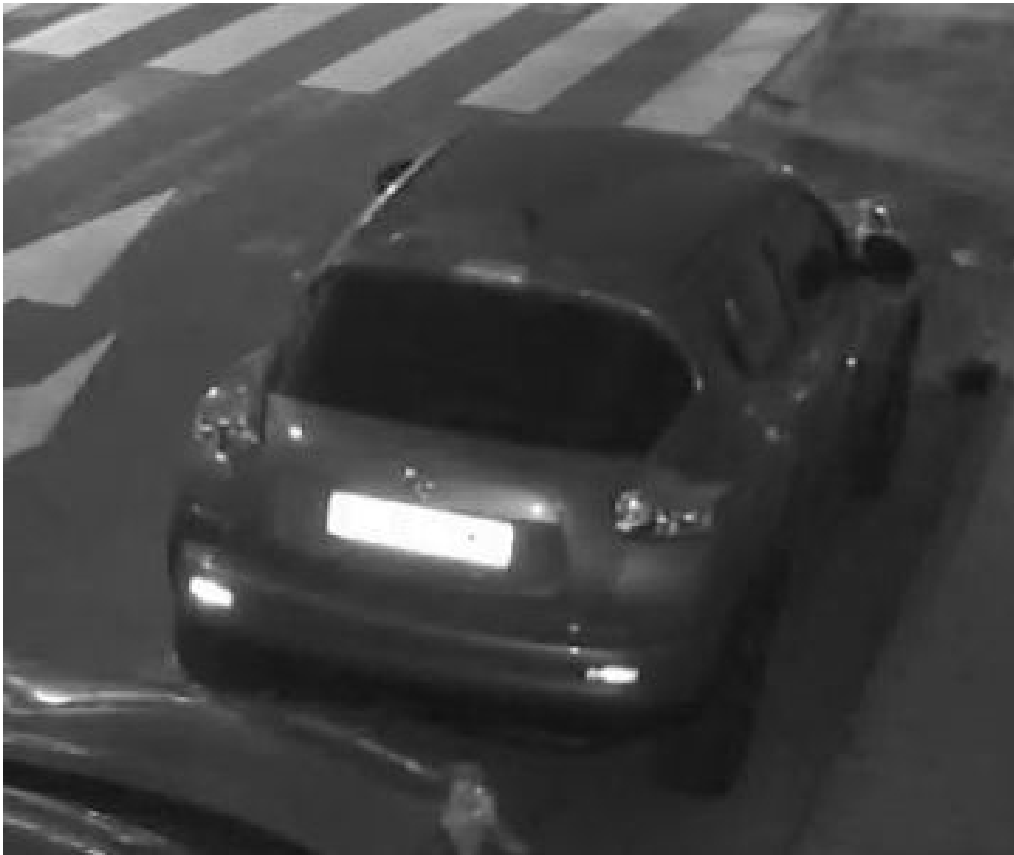
Fig. 16: Over exposed license plates due to too strong IR LED light
