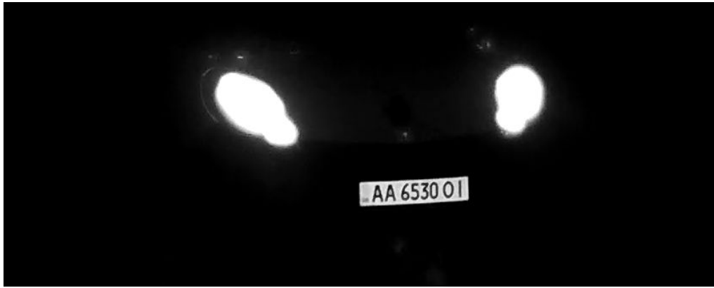
Fig. 10: Easily readable license plate at night with infrared LED illumination
