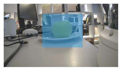
A privacy zone masks a defined image area to protect privacy. It applies to all streams, the recording and the live view and has no influence on analysis functions such as motion detection. You can define up to 8 different privacy zones. After setting up a privacy zone, a frame is displayed in the live view, the color, size and position of which can be adjusted.
