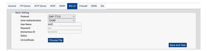
IEEE 802.1X is a standard for authentication in computer networks and defines the encapsulation of the Extensible Authentication Protocol (EAP) via IEEE 802.
