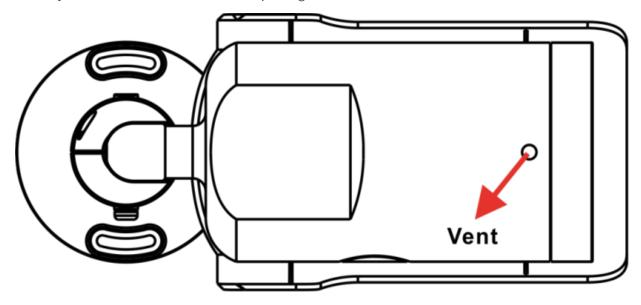
**CAUTION!** Removing the desiccants package will activate the venting system and humidity can enter the camera housing if the camera is not powered up immediately after installing!
