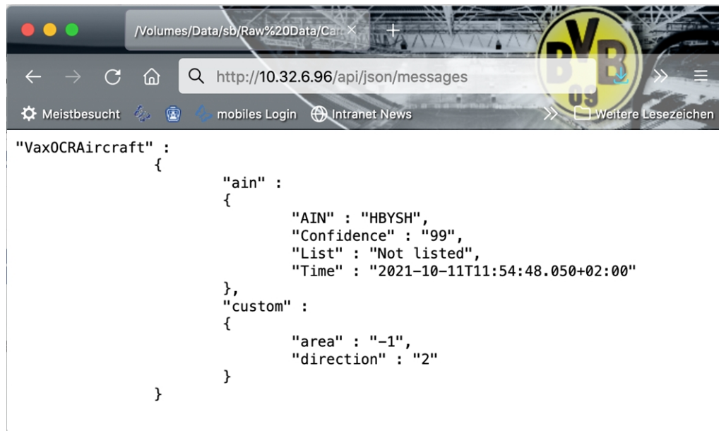
Fig. 8: Example: Meta data transmitted within a MxMessage of the Vaxtor Aircraft Identification Number Recognition App
