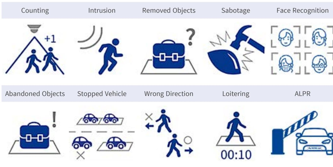
The latest computer vision technology makes the DNN-accelerated video processing engine efficient at the edge. This integrated engine provides high accuracy, and 10 (DNN-based) video analytics functions including ALPR and human face recognition. Moreover, it allows simultaneous detection on multiple objects.
