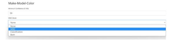
When MMC is enabled, the engine will find a plate and the MMC analytic will attempt to identify the make model and, if possible, the color of the vehicle using Deep Learning technology.
