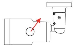
2. Open up the internal cover using a security Torx.
