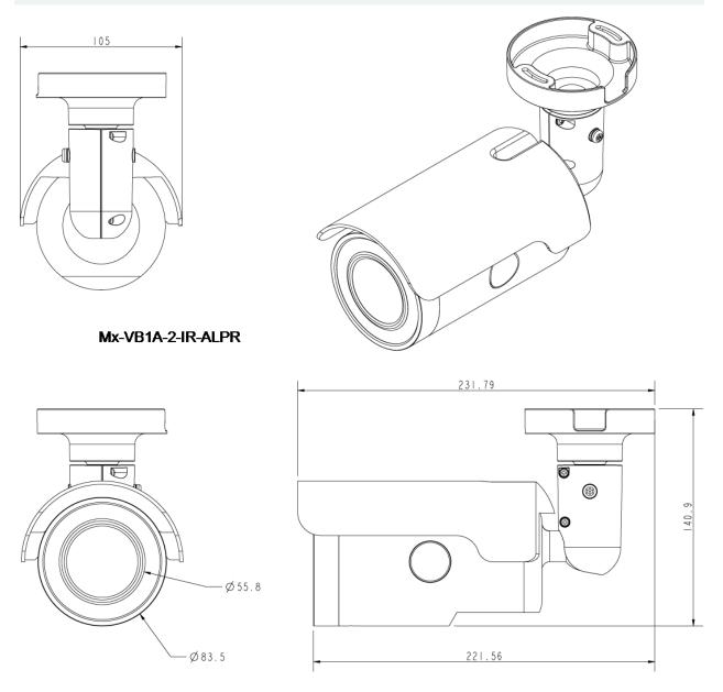
Fig. 1: Mx-VB1A-2-IR-ALPR: All measurements in mm
