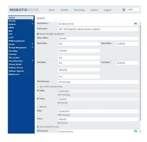
Here we can set the time zone and synchronize the time with a time server and in this example, we are using one of the UK NTP Servers.
