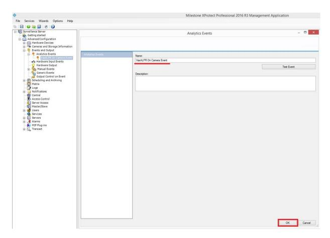
Fig. 7: Surveillance Server > Advanced Configuration > Events and Output > Analytic Events: ALPR Event
