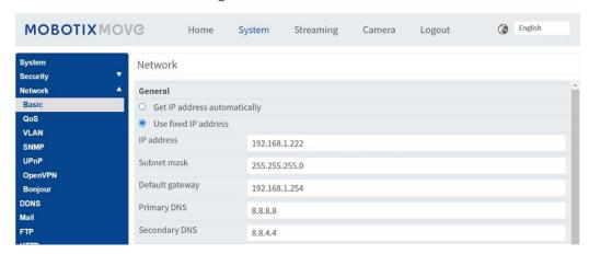
In this case Google's is 8.8.8.8 with a secondary server of 8.8.4.4. These are free Google DNS servers which will map any domain names needed to the correct IP address.
