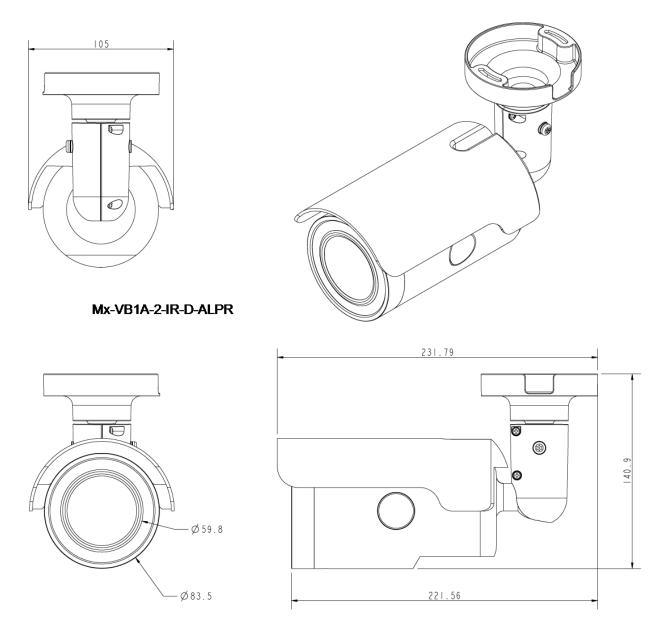
Fig. 2: Mx-VB1A-2-IR-D-ALPR: All measurements in mm
