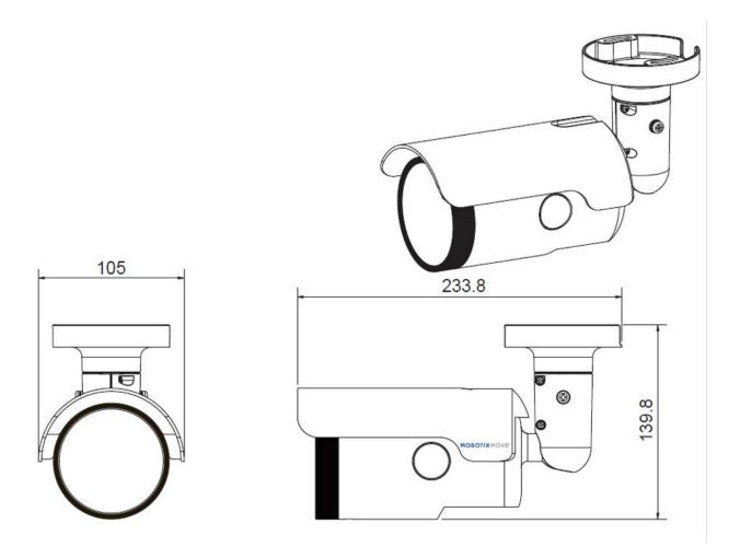
Fig. 1: Mx-VB1A-8-IR-VA: All measurements in mm
