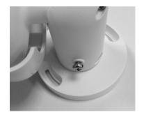
2. If the screw holes are blocked by the camera body, loosen the screw shown in the right figure but do not detach it. Then rotate the camera body to reach the screw holes.
