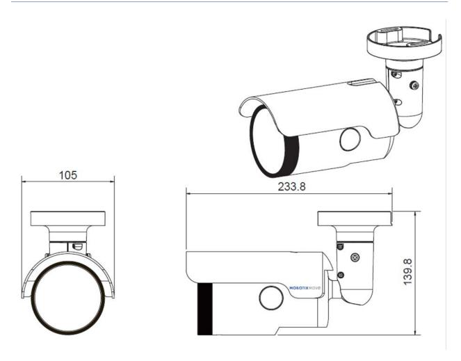
Fig. 1: Mx-VB3A-2-IR-VA: All measurements in mm
