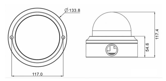
Fig. 1: Mx-VD1A-8-IR-VA: All measurements in mm
