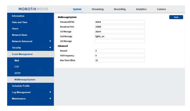
The camera can send notifications via the MxMessageSystem by triggered events.
