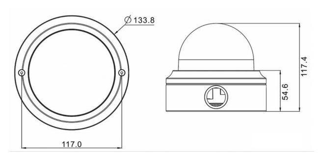
Fig. 1: Mx-VD2A-5-IR-VA: All measurements in mm
