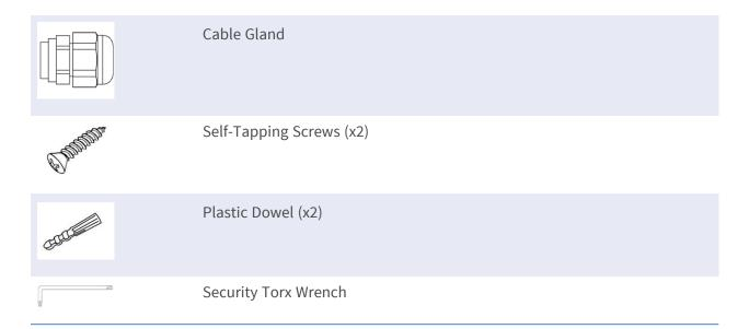
**NOTE!** The supplied self-tapping screws are for soft substances/materials such as wood. For other installation environments, such as solid or sheet rock walls, users **MUST** pre-drill and use plastic dowels before fastening the camera onto the wall.
