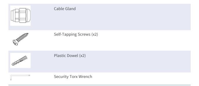
**NOTE!** The supplied self-tapping screws are for soft substances/materials such as wood. For other installation environments, such as solid or sheet rock walls, users **MUST** pre-drill and use plastic dowels before fastening the camera onto the wall.
