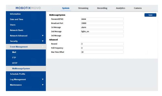
The camera can send notifications via the MxMessageSystem by triggered events.
