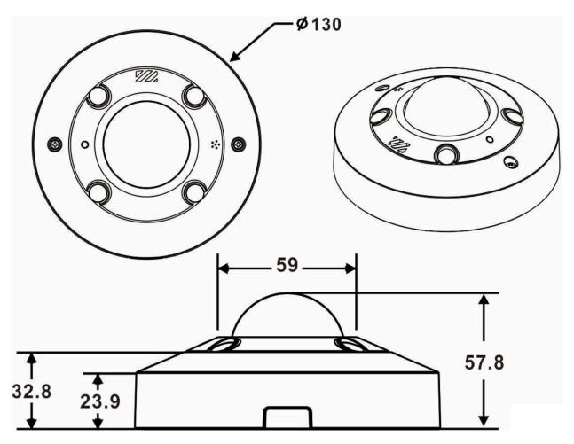
Fig. 1: Mx-VH1A-12-IR-VA: All measurements in mm
