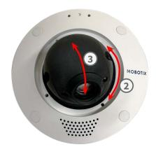
**CAUTION!** Never use force when adjusting the direction of the camera, as this could damage the camera beyond repair.
