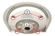
Use two short allen screws W.4, p. 22 with one washer W.6, p. 22 each to secure the camera on the rear side of the bottom plate ①.
