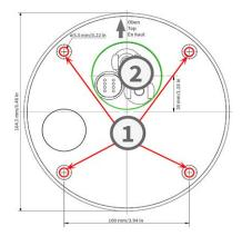
**NOTE!** The drilling template also includes a circle ② marking the minimum size and position of the wall outlet, in addition to the drilling holes.
