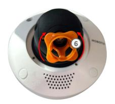
**NOTE!** After focusing, further adjustment of the focusing must be made due to the optical properties of the dome.
