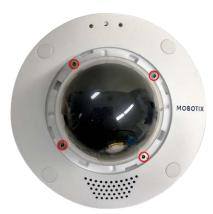
3. Pull the dome off upwards.
