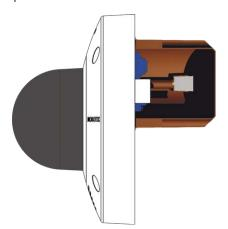
Before mounting the camera, make sure that a network connection with power supply according to the PoE Plus (802.3at-2009) standard is available at the mounting position (see Connecting the Camera, p. 1).
