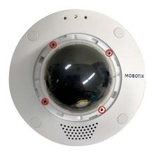
2. Attach the cover of the clamping ring ① by turning clockwise until resistance is felt.
