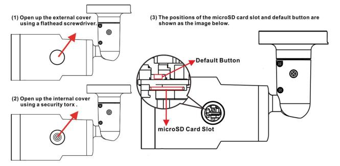
The positions of microSD card slot and reset button are shown below.
