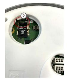
Unlock the microSD card holder: Flip up the metal cover ② of microSD card (e.g. with a fingernail).
