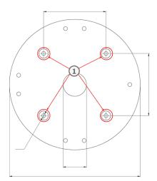
If you If you use the 0° set, close the cable openings ② that are not needed with the enclosed closing plugs. Fix each of them in place from the inside using a small hexagonal nut.
