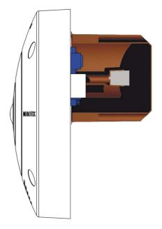
Before mounting the camera, make sure that a network connection with power supply according to the PoE Plus (802.3at-2009) standard is available at the mounting position (see Connecting the Camera, p. 1).
