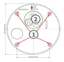
**NOTE!** The drilling template also includes a circle ② marking the minimum size and position of the wall outlet, in addition to the drilling holes.
