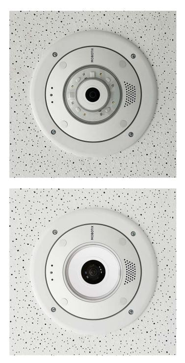
**CAUTION!** Before mounting the camera, make sure that a network connection with power supply according to the PoE Plus (802.3at-2009) standard is available at the mounting position (see Connecting the Camera to the Network).
