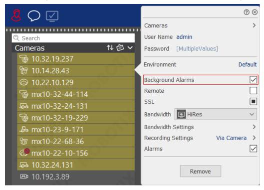
Fig. 61: Bulk configuration of multiple cameras
