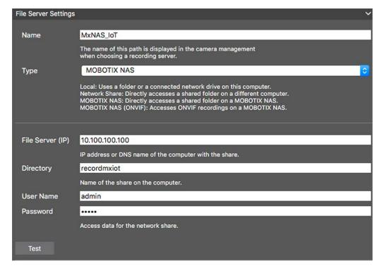
File Server (IP): IP address or DNS name and port of the MOBOTIX NAS.
