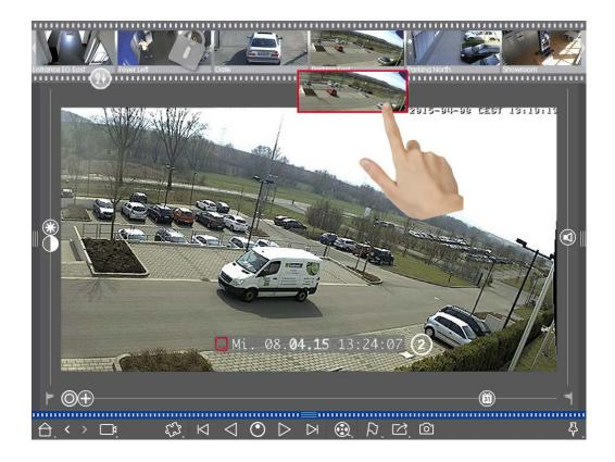
5. The playback automatically selects the recording that follows the end of camera A's recording ② . You can continue this process for any number of cameras.
