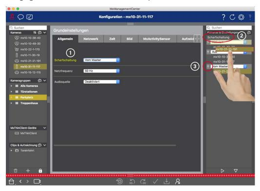
Fig. 23: Changing a value for one camera or for multiple cameras
