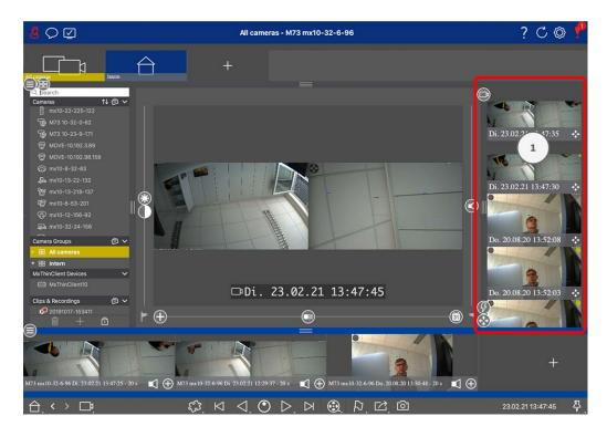
The Alarm Bar ① is located at the **right** of MxManagementCenter. It turns red when there is an unacknowledged alarm event. This happens only if the **Alarms** option has been activated in the Camera Configuration dialog box and if the event types responsible for triggering an alarm have been activated.
