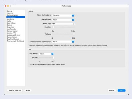
Camera icon and group icon in the Graphic view In order for the camera icon and group icon to turn red or green in the Graphics view when an alarm event occurs, the same settings must be made as for notification in the Alarm bar and Alarm Info bar.
