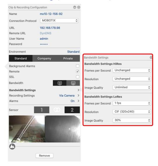
Fig. 64: Bandwidth Settings (MOBOTIX Cameras)
