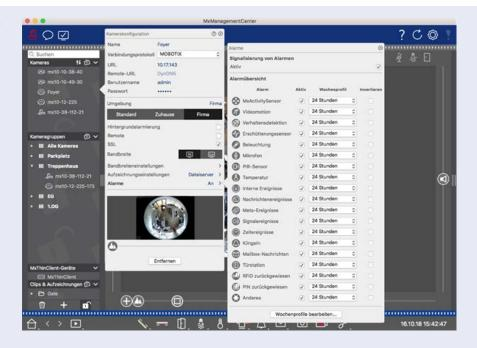
In addition, you can select a weekly profile for every event type that should trigger an alarm.
