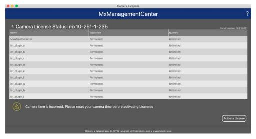
**NOTE!** If necessary, correct the time set on the camera.
