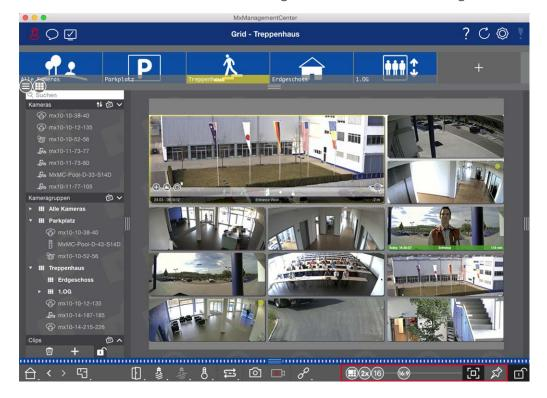
Fig. 35: Setting the layout for the Grid View
