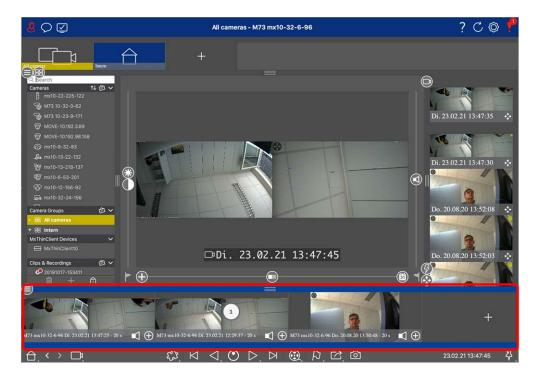
The Export Bar ① is located at the **bottom** of the MxManagementCenter. It contains the The Histogram Bar, p. 294 which visualizes the distribution of event frequency.
