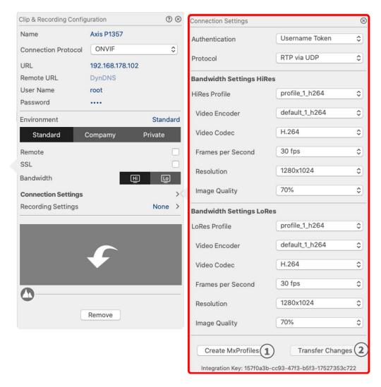
Fig. 65: Connection Settings (MOBOTIX MOVE/ONVIF-S/G Cameras)
