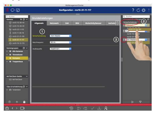
Fig. 158: Changing a value for one camera or for multiple cameras
