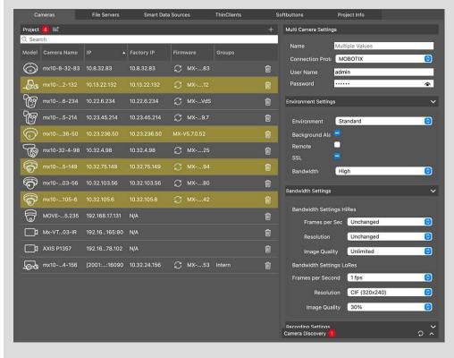
Fig. 95: Bulk configuration of multiple cameras
