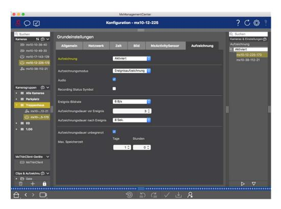
**Arming:** The arming feature for event control handles camera recording. However, the main arming of the camera needs to be activated in order to make the recordings in the first place.
