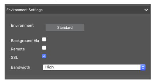
**Environment**: Shows the current network environment. After starting the program for the first time, it shows the standard environment. All existing network environments are shown in the blue bar. Click on the environment you want to use and enter the network settings for this environment. To define environments, see Network Environments, p. 125.
