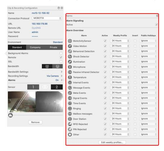
Fig. 29: Setting Alarm Filters
