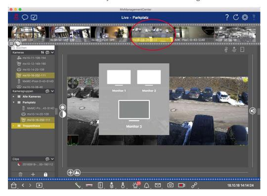
Fig. 123: Displaying Live Images On Monitors Connected To The Computer
