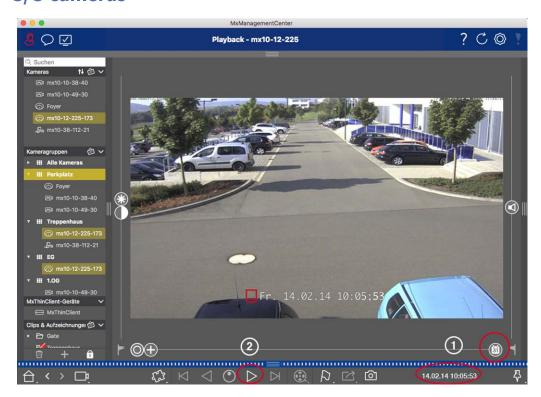
Fig. 127: General operation of the Playback View for MOBOTIX MOVE and ONVIF-S/G cameras
