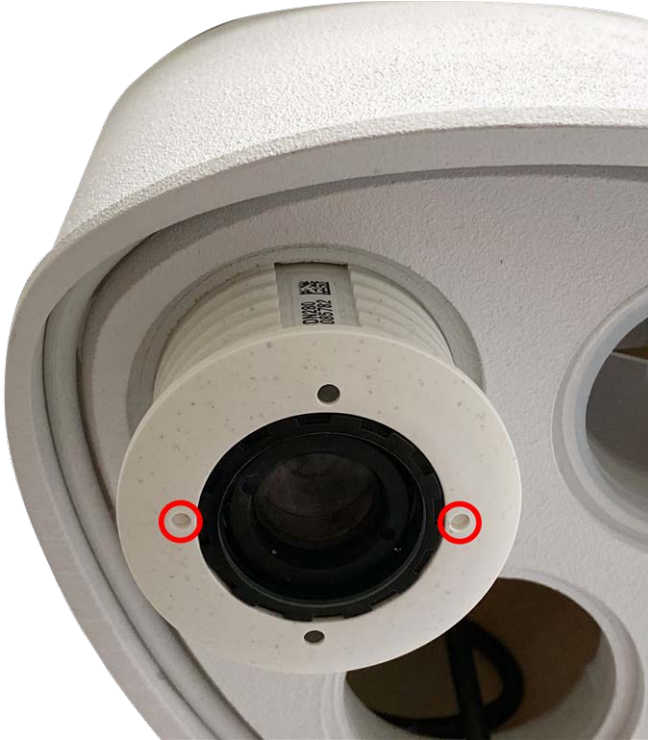
Fig. 9: Unlock the sensor module
