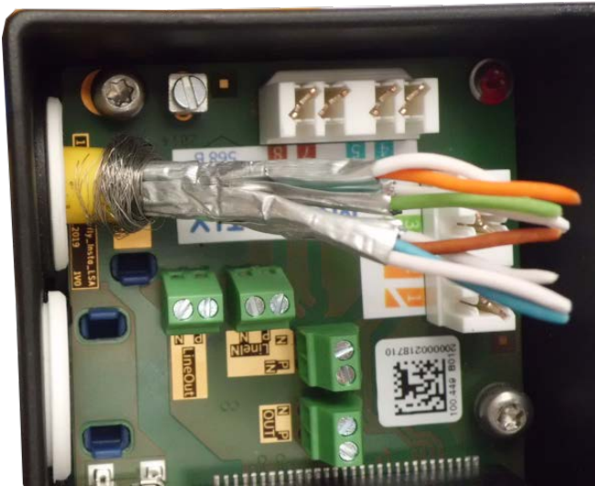
Fig. 23: Network cable inserted, plug properly seated
