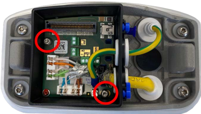
Fig. 30: Mount the Connector Box LSA (top view) using the two screws (highlighted red in the figure) on the mounting plate
