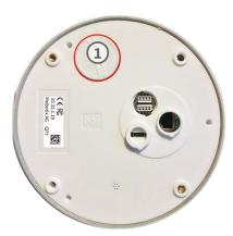
3. **Unlock the microSD card holder:** Flip up the metal cover ② of microSD card (e.g. with a fingernail).
