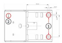
2. Drill the holes with a 10 mm wall drill then place the included dowels in the drilled holes.
