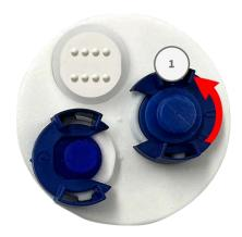
2. Plug the supplied patch cable ② into the network connector and press the plug in firmly until the blue sealing ring clicks into place.
