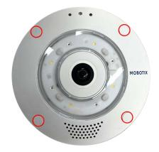
9. Using the supplied Allen wrench W.2, p. 22, secure the camera to the bottom plate of the On-Wall Set with four Allen screws W.5, p. 22 and one washer W.6, p. 22 each.
