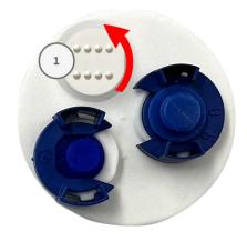
2. Insert the cables of the I/O devices through the openings provided in the dome cap.
