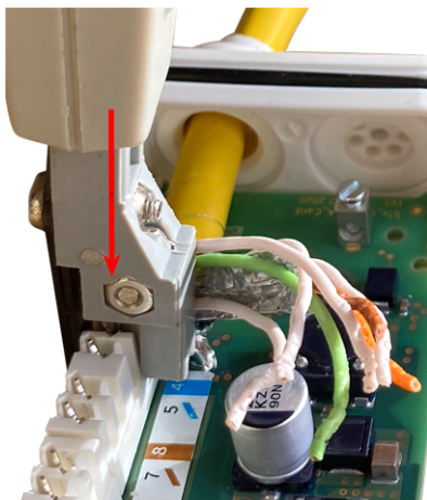
Fig. 13: Network wires connected using LSA+/Krone tool
