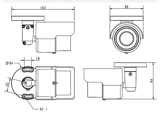
Fig. 1: Mx-BC2A-2-IR: All measurements in mm
