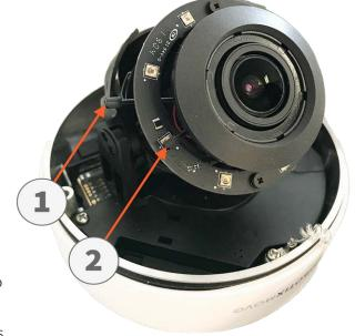
**NOTE!** Take care to properly tighten the focal length lever ①, the focus lever ②, and the screws of the 3-axis gimbal to prevent unwanted changes due to vibration, for example.
