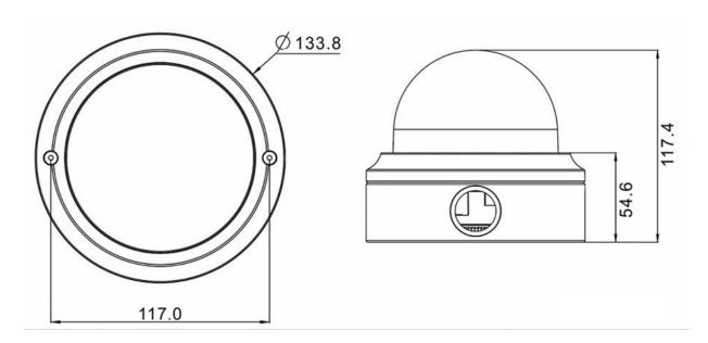
Fig. 1: Mx-VD2A-2-IR: All measurements in mm
