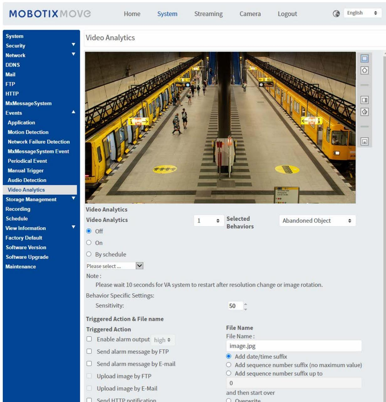
The screenshot shows the MOBOTIXMOVE web interface. The top navigation bar includes 'Home', 'System', 'Streaming', 'Camera', and 'Logout'. The left sidebar menu is expanded to 'Video Analytics'. The main content area is titled 'Video Analytics' and features a video feed of a train station platform. Below the video feed, the configuration options are as follows:
