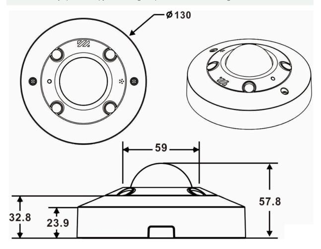
Fig. 1: Mx-VH1A-12-IR-VA: All measurements in mm
