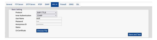
IEEE 802.1X is a standard for authentication in computer networks and defines the encapsulation of the Extensible Authentication Protocol (EAP) via IEEE 802.
