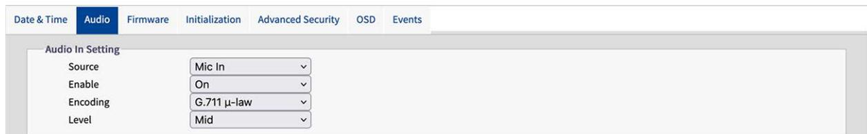
The screenshot shows the 'Audio In Setting' configuration page. It features a navigation bar with tabs for 'Date & Time', 'Audio', 'Firmware', 'Initialization', 'Advanced Security', 'OSD', and 'Events'. The 'Audio' tab is selected. Below the navigation bar, there is a section titled 'Audio In Setting' with four configuration items, each with a dropdown menu:
