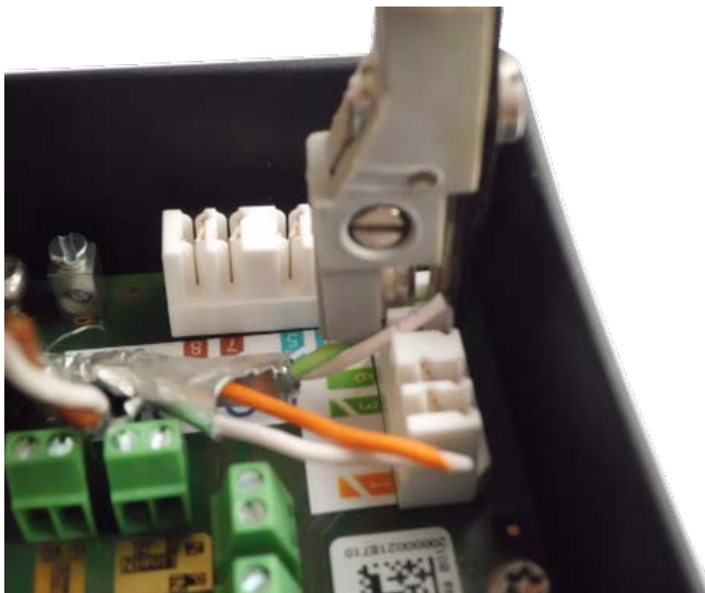
Fig. 26: Network wires connected using LSA+/Krone tool
