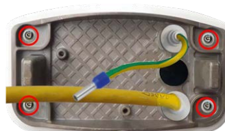
Fig. 17: Installed and ready for Connector Box LSA
