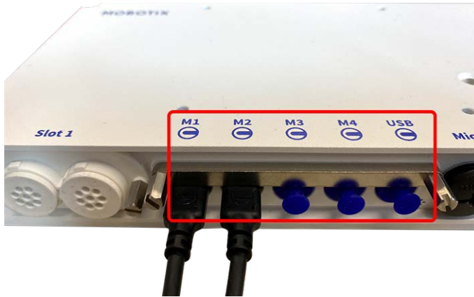
Fig. 3: 4 Module Connector Ports and 1 USB-C interface
