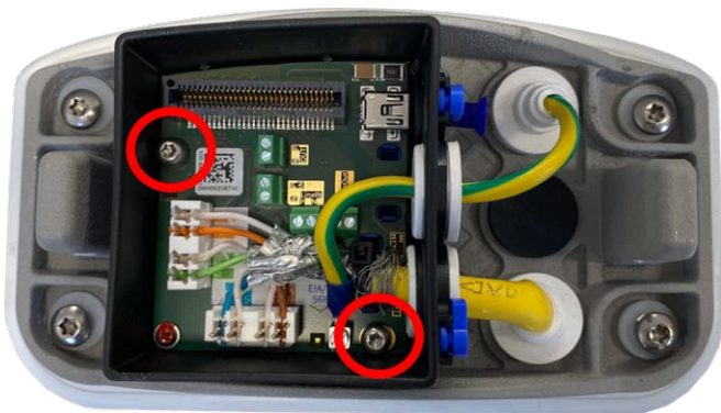
Fig. 31: Mount the Connector Box LSA (top view) using the two screws (highlighted red in the figure) on the mounting plate
