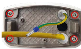
Fig. 12: Installed and ready for Connector Box LSA
