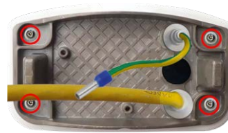
Fig. 18: Installed and ready for Connector Box LSA
