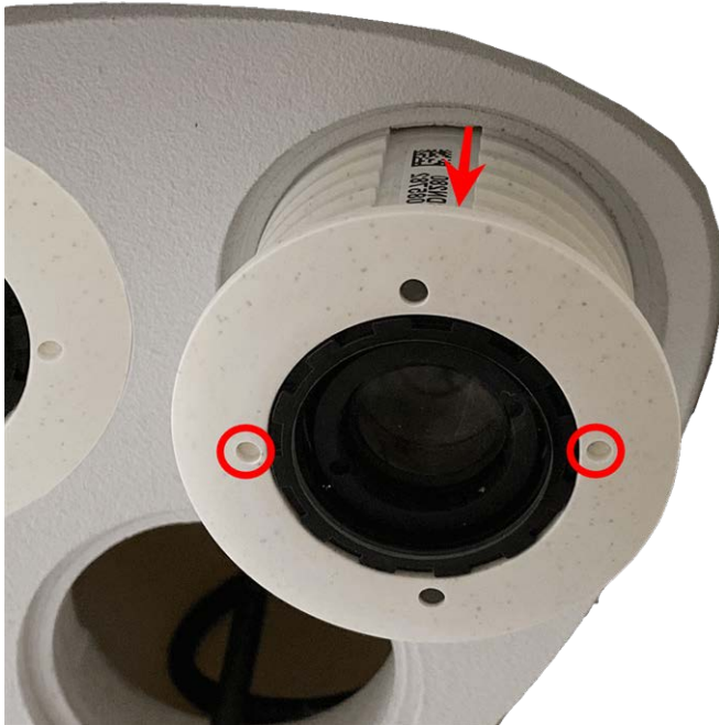
Fig. 10: Remove sensor module from the module housing
