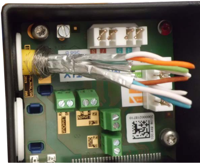
Fig. 24: Network cable inserted, plug properly seated
