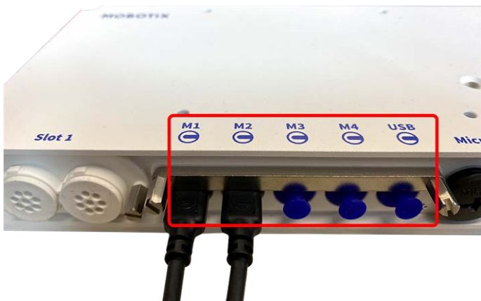
Fig. 8: 4 Module Connector Ports and 1 USB-C interface
