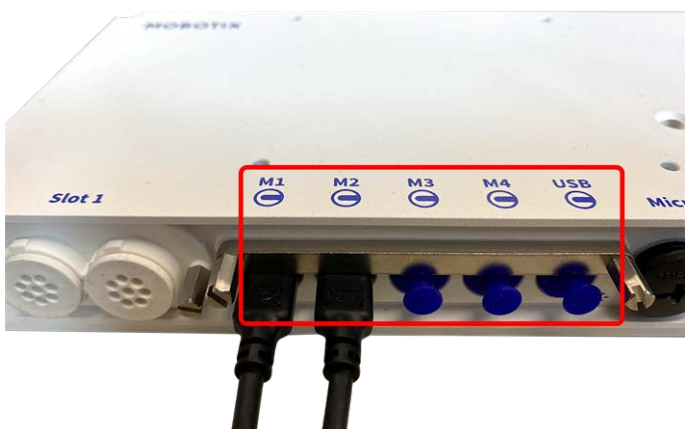
Fig. 8: 4 Module Connector Ports and 1 USB-C interface
