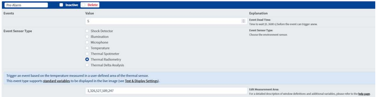
Fig. 6: Pre-Alarm radiometry event profile with measurement area.
