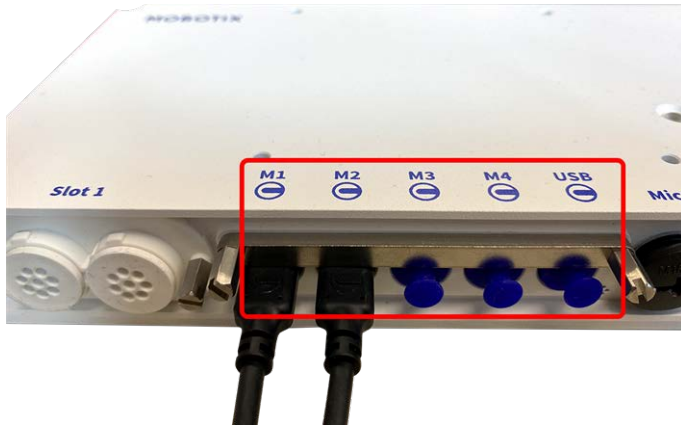
Fig. 3: 4 Module Connector Ports and 1 USB-C interface
