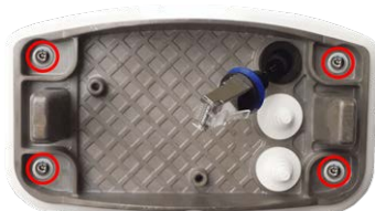
Fig. 6: Installed and ready for Connector Box RJ45
