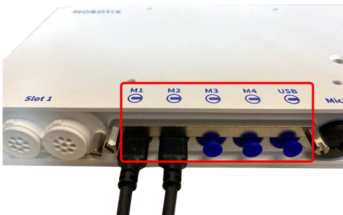
Fig. 5: 4 Module Connector Ports and 1 USB-C interface
