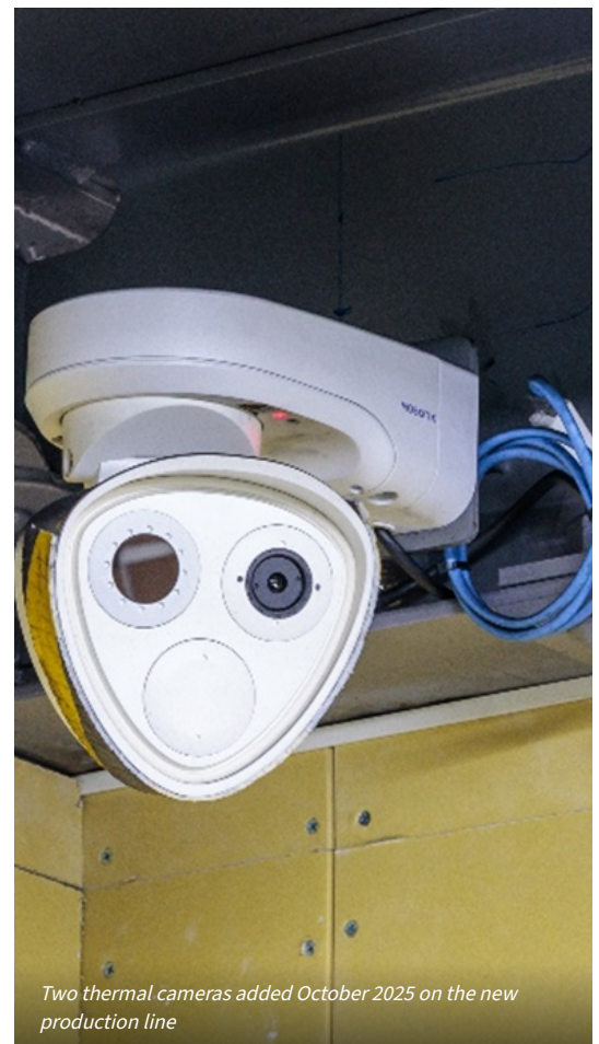
Thermal and visible footage recorded simultaneously — a false alarm is confirmed at a glance
