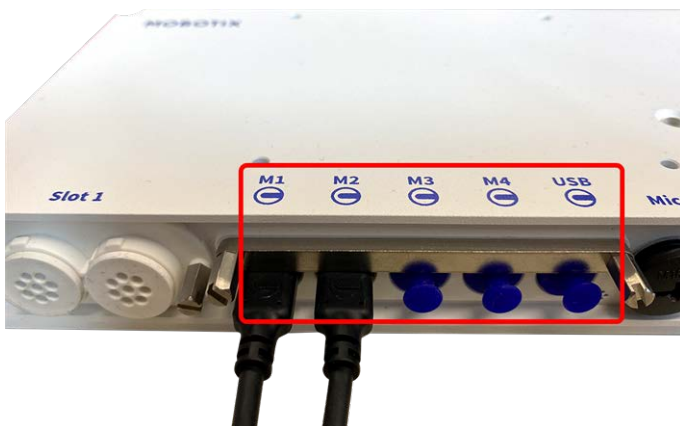
Fig. 5: 4 Module Connector Ports and 1 USB-C interface
