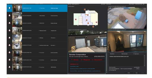
Symphony VMS displaying access control events within its Alarm Console. Alarms appear in the alarm log as well as on a graphical map.
