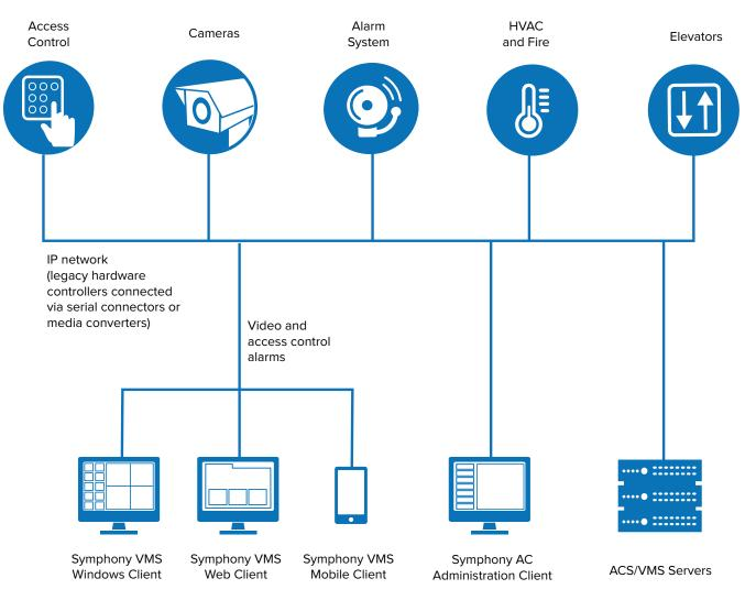
Sample deployment with integrated access control and video
