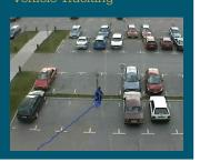
Detect and track moving objects and classify them as a person, vehicle, or unknown. Movement tracks are recorded to know exactly where each object came from and where it left the camera's point-of-view.
